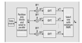
Fig. 1. SLM Block Diagram.
