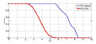
Fig. 3. Comparison Graphs of CCDF and PAPR Using RS Clipping and RS SLM.
